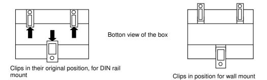
Use the holes of the clips to fix the box in the wall using screws. Use the template below for the wall holes.
